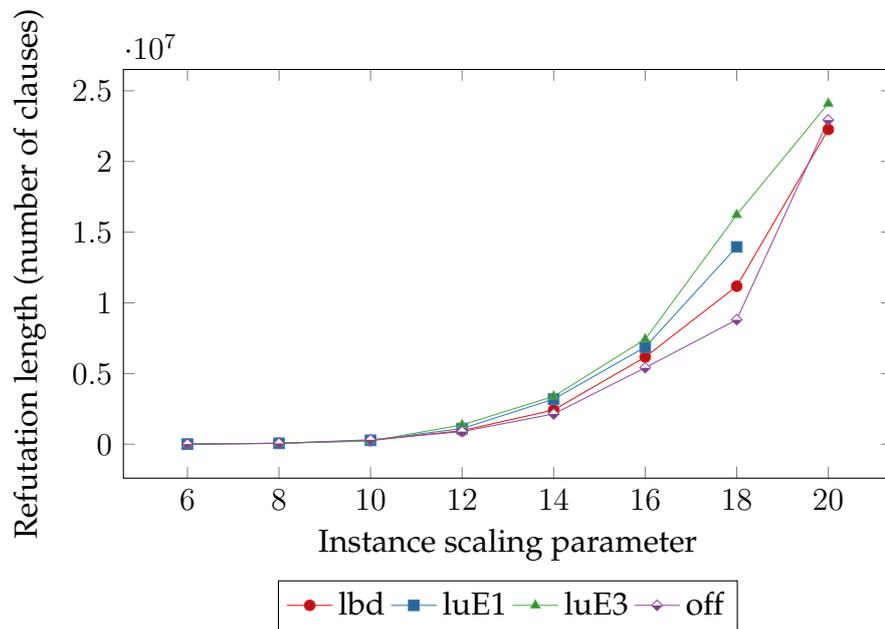
Figure A.17: The effects of restarts on refutation length, rphp\_5 formulae (recursive minimization, unit elimination mode "1", lin clause erasure)
