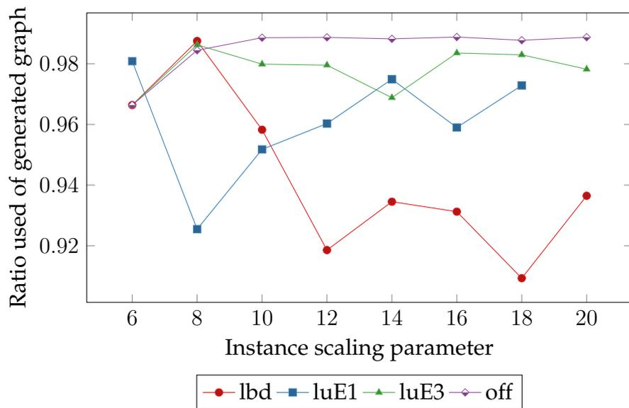
Figure A.27: The effects of restarts on ratio of generated graph being used as proof, rphp\_5 formulae (recursive minimization, unit elimination mode "1", lin clause erasure). The ratio refers to  $\frac{\text{Number of vertices in refutation}}{\text{Number of vertices in full graph}}$
